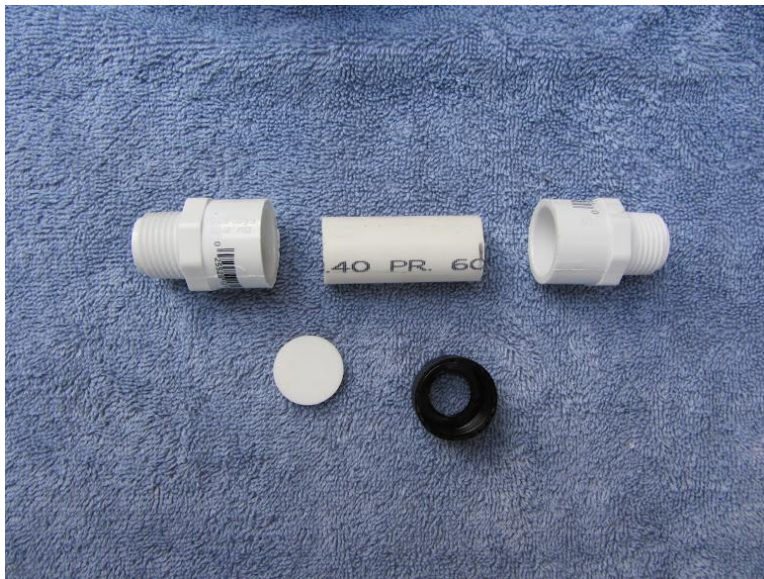
Figure 3: Components of extraction port for each reactor showing (1) two hybrid treaded/non-threaded PVC-connectors (top left/right), (2) one four inch length of ½”-(OD) PVC-piping (top middle) and (3) one ½”-(OD) silicone septum (bottom left). Silicon septum were placed on one end of the PVC-piping and inserted into the non-threaded side of one connector to allow syringe extraction.
