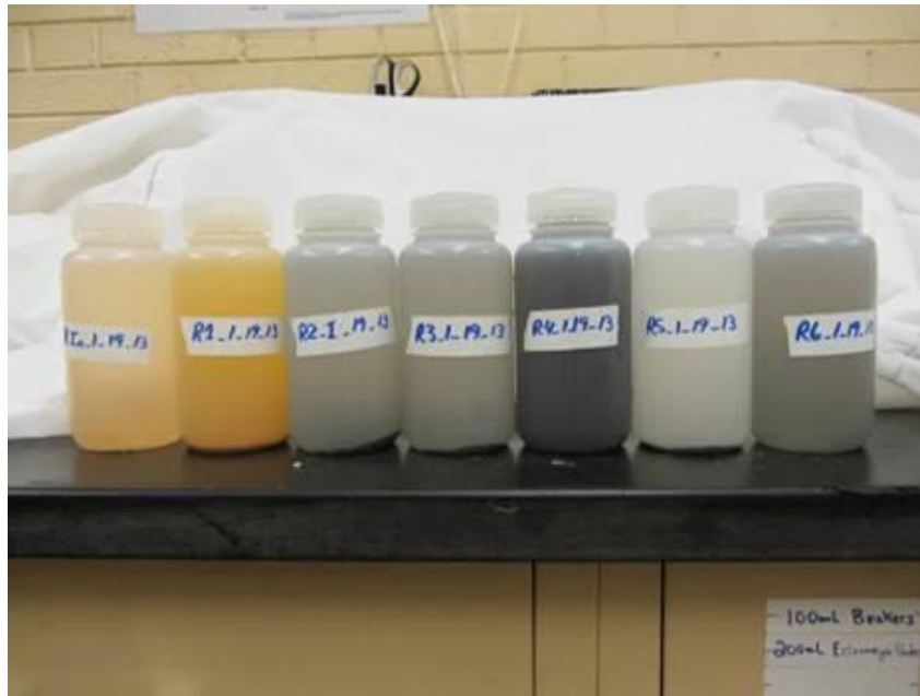
Figure 45: Photograph of samples within 1 hour of collection from left to right samples contain influent AMD, limestone only (R1) and bioreactor effluent (R2-R6).
