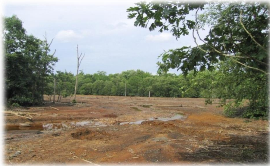
Figure 1: Photograph of acidic iron oxide (Ochre) sediment deposited at the Tab-Simco AML site in southern Illinois. View is taken in a north-easterly direction from the location of the main AMD seep. (Photo taken by Behum, 2004)
