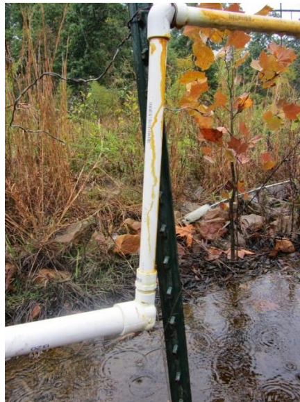
Figure 6: Photograph of 1''-1/2'' (ID) elbow reducing connector added prior to reactor test-cells to decrease flow-path volume and increase flow-rate upwards to provide the additional height required to gravitationally feed each reactor AMD influent.
